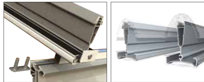
A twin bolt slides into the captivated bolt slot in the eaves beam, prior to the glazing bar being tightened down.
