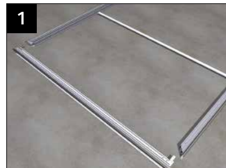
Layout the pieces of the lantern eaves beam.
