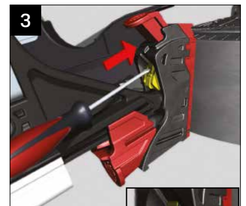
3 Insert the 5mm wide flat blade screwdriver and gently push against the upper edge of the roller cam (marked yellow).
