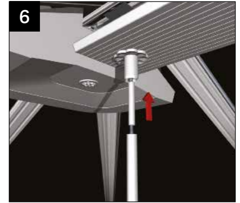
6 Now cut the PVCu conduit to length, taking care to make allowances for its inset into both the bracket and boss. Take the piece of vertical pvc conduit and slide over the threaded bar and push it home into the ridge cover.
