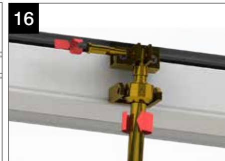
16 Attach the winder head to the sash bracket, using the plunger pin. Hold the winder at the relevant angle. Turn the winder body clockwise until it locks with the sash bracket.
