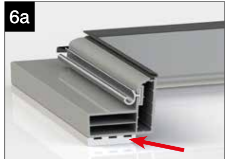
6a If existing glazing is 32/35mm a packer will have been pre-fitted to the frame.
