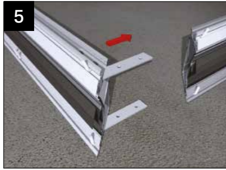
5 Slide the cleated corners into the adjacent piece of pagoda beam.
