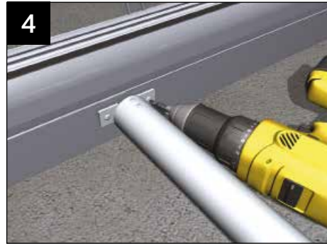
4 Attach the strut at the mid point of the long sides.
