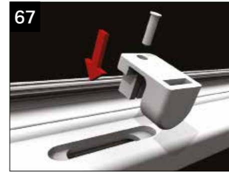
67 Ensure the ventilation button is fixed into the ridge undercladding as shown before you install the cladding.
